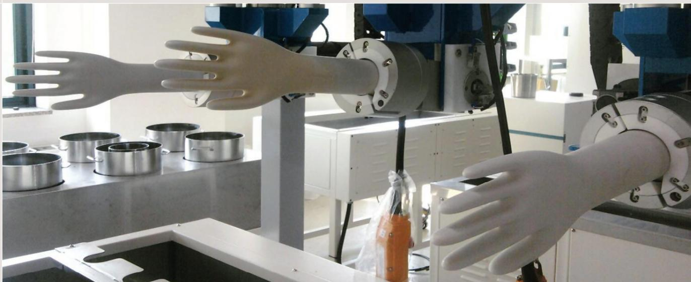
Whole dipping process proceeded by Dipping Instrument of
